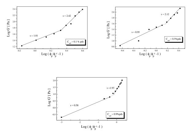
**Fig.3.** Critical exposants for G'~( $\phi_p/\phi_p^c$ -1) for given salt concentration
