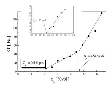
**Fig.3.** Determination of a critical volume fraction  $\Phi^{p}_{c}$  and Ppt for different concentrations in salt
