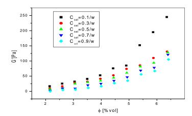
Fig.2. Evolution of elastic modulus G' vs the volume fraction
