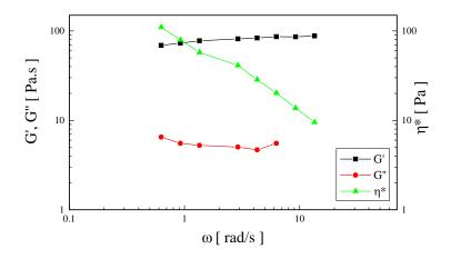
**Fig.1.** Dynamic Response of clays dispersions for  $\gamma = 0.025$ , C<sub>sel</sub> =0.5% w/w, C<sub>ben</sub>=12% w/w
