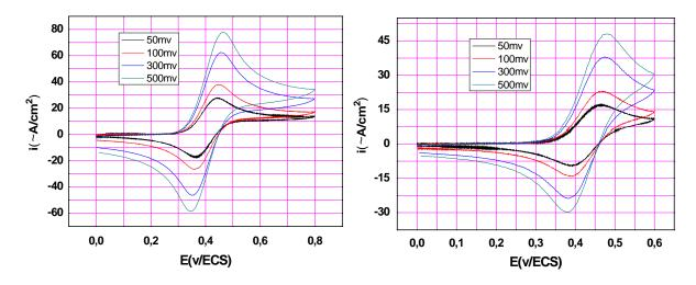
**Fig.5.** cyclic voltammetry of ferrocene and compound **3** 1mM and 100 mM Bu<sub>4</sub>NBF<sub>4</sub> in CH<sub>3</sub>CN at 2 mm diameter glassy carbon working electrode, Pt counter electrode, and CSE reference electrode at (0.05, 0.10, 0.30, 0.50 V.s<sup>-1</sup>).
