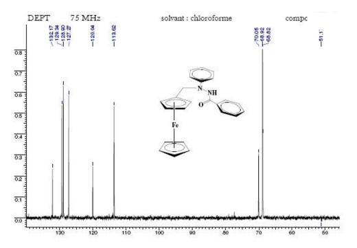
Fig.3. Dept spectrum of N'-Ferrocenylmethyl-N'-Phenylbenzohydrazide in CDCl<sub>3</sub>
