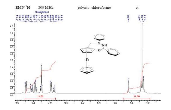
Fig.1.<sup>1</sup>H. N.M.R spectrum of N'-Ferrocenylmethyl-N'-Phenylbenzohydrazide in CDCl<sub>3</sub>
