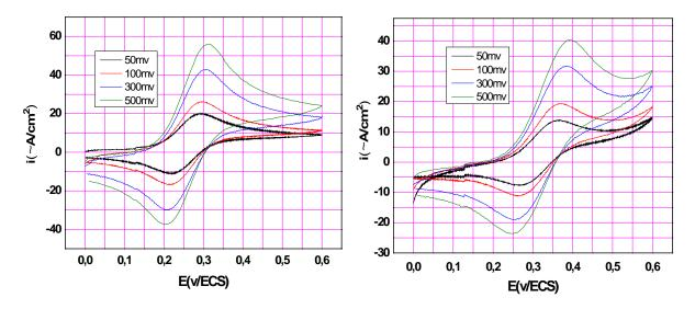
Fig.6. cyclic voltammetry of ferrocene and compound 3 2mM in ethanol/aq.H<sub>2</sub>SO<sub>4</sub> at 2 mm diameter glassy carbon working electrode, Pt counter electrode, and CSE reference electrode at  $(0.05, 0.10, 0.30, 0.50 \text{ V.s}^{-1})$ .
