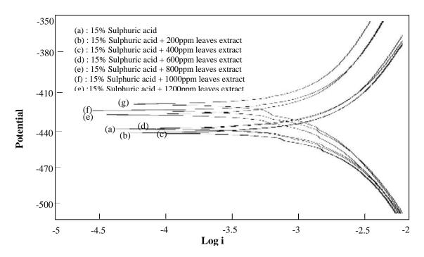
Fig.3. Polarization curves of mild steel in 15% H<sub>2</sub>SO<sub>4</sub> solution devoid and containing different concentrations of leaves extract.
