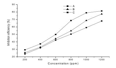
**Fig.1.** variation of the inhibition efficiency with plant concentrations A: leaves extract, B: stems extract, C: flowers extract.
