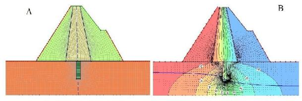
Structure gridding of Badf dam with cutoff wall at a depth of 25 m
