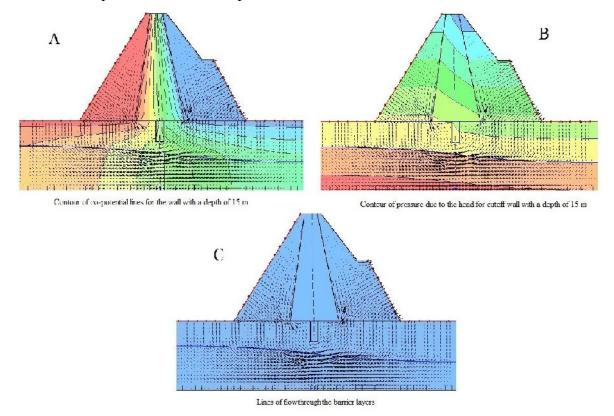
**Fig.1.** Schematic figures for contours of co-potential lines (A), head pressure (B) and flow through lines (C) for different parts of dam at a depth of 15 meters
