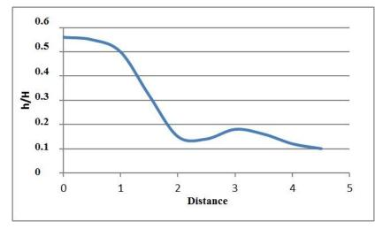
Fig.6. Reduced uplift pressure in the presence of cutoff wall at the sides
