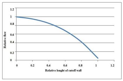
Fig.5. Diagram of relative flow-through rate based on the relative length of cutoff wall
