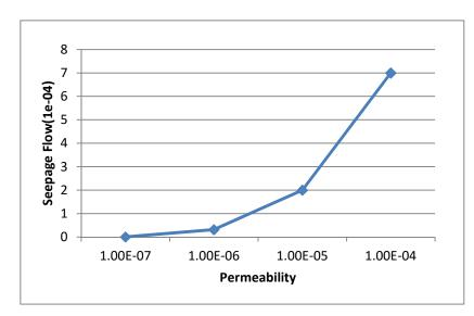
Fig.4. Effect of soil permeability on the rate of seepage flow from the middle section of dam
