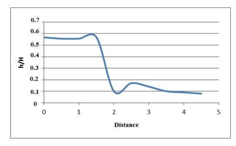
Fig.7. Reduced uplift pressure with cutoff wall in the middle
