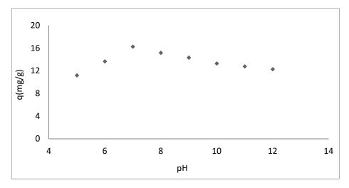
Fig.6. Effect of pH on the surface adsorption of nitrate on LDH
