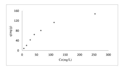
Fig.8. Isotherm of nitrate adsorption on LDH
