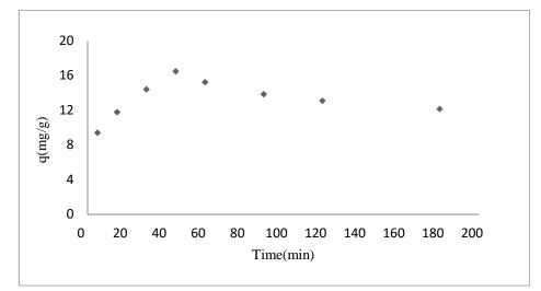
Fig.4. Effect of contact time on the surface adsorption of nitrate on LDH
