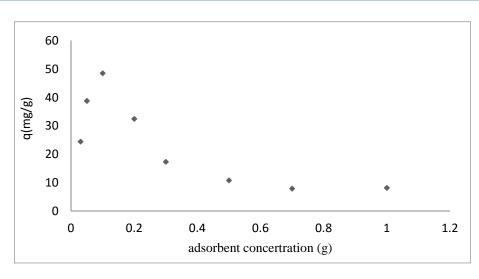
Fig.7. Adsorbent concentration on the surface adsorption of nitrate on LDH
