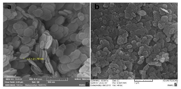
Fig.1. Scanning electron microscopic image for manufactured chloride-LDH
