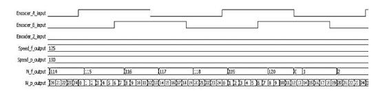
Fig.11. Simulation result of Verilog code for speed computing block in high speed range
