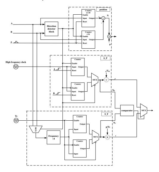
Fig.4. Hardware structure of proposed Encoder Processing Unit
