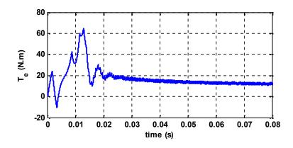
Fig.9. Electromagnetic torque waveform
