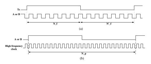
Fig.3. Methods of speed calculation a. based on frequency b. based on period
