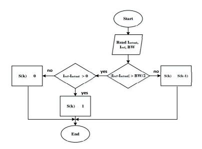
Fig.7. Flowchart of hysteresis band controller
