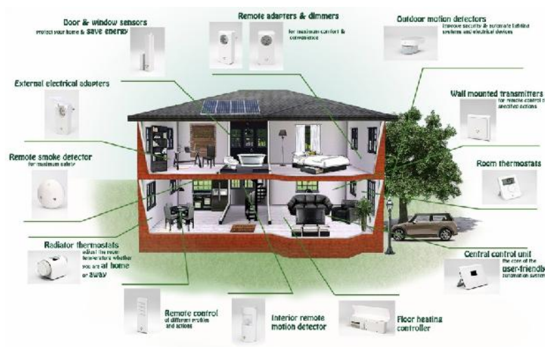
Fig.1. How to implement BMS and associated components with each other inside the building
