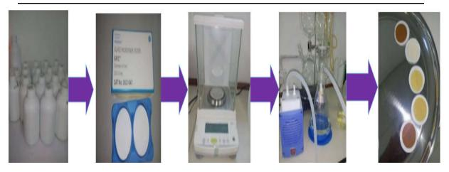
Fig.2. a) Sample water b) Membrane filter c) Electronic weighing d) Filtration apparatus
