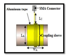
Fig. 2. Coupling sleeve structure.
