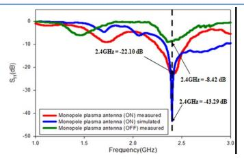
**Fig.5.** Simulated and measured reflection coefficient,  $S_{11}$  for monopole plasma antenna.
