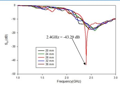
**Fig.4.** The effects on reflection coefficient,  $S_{11}$  due to change of the diameter of plasma antenna.
