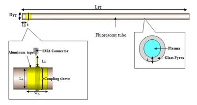
Fig.1. The structure of a monopole plasma antenna.
