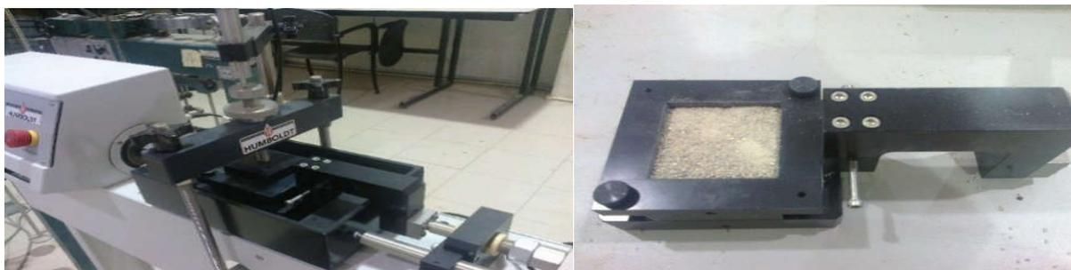
**Fig.2.** Shear box test for EPS-sand mixture
