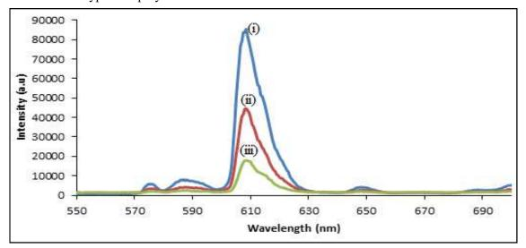
Fig.1.Emission spectra of (i) PVK, (ii) PVK:PVDF-HfP, and (iii) PVK:PVP blend with EuDBMPhen
