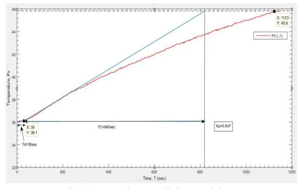
Fig.5. Process reaction curve with thermocouple input
