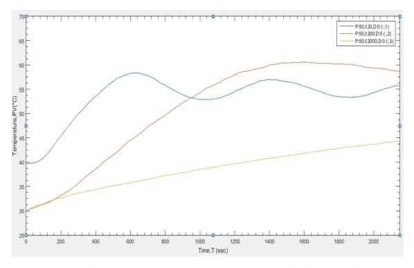
Fig.16.Effect on temperature measured using thermocouple with change of T<sub>I</sub>
