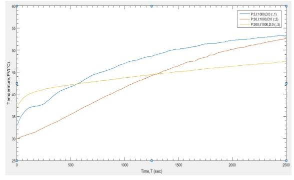
Fig.15.Effect on temperature measured using thermocouple with change of proportional band
