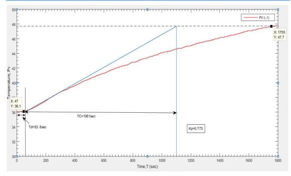
Fig.4. Process reaction curve with RTD input
