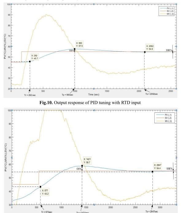
Fig.11. Output response of PID tuning with thermocouple input
