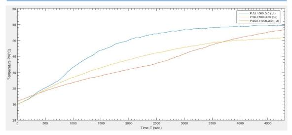
Fig.12. Effect on temperature measured using RTD with change of proportional band
