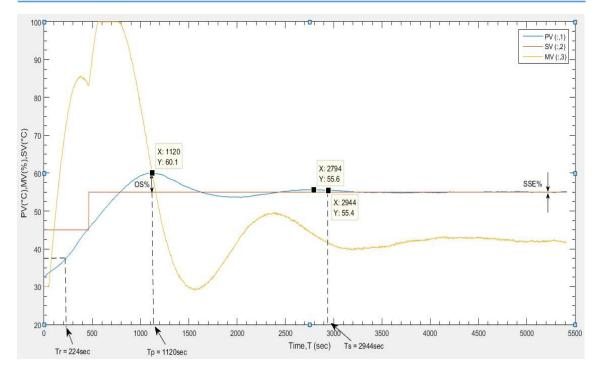
Fig.9. Closed-loop response of PID tuning with thermocouple input
