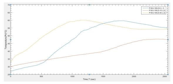
Fig.14. Effect on temperature measured using RTD with change of  $T_D$
