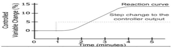
Fig.3.Process reaction curve foropen-loop response [17]
