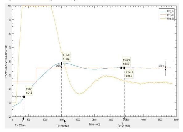
Fig.8. Closed-loop response of PID tuning with RTD input
