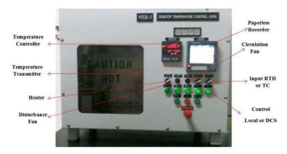
Fig.1. Temperature control plant [13]
