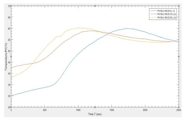
Fig.17.Effect on temperature measured using thermocouple with change of  $T_D$ In addition, Table 9 shows the changes of tuning values that affect temperature measurement through use of thermocouple sensor.
