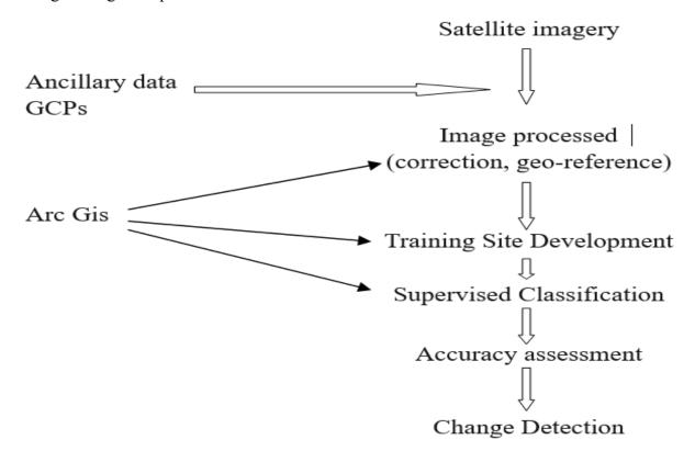
Fig.2. The LULC flowchart image processing procedures
