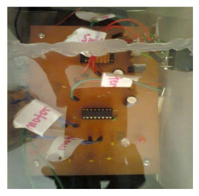
Fig.5. H-bridge on the PCB board
