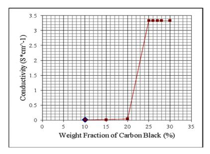
Fig.3. Conductivity of nanocomposites with CB loading
