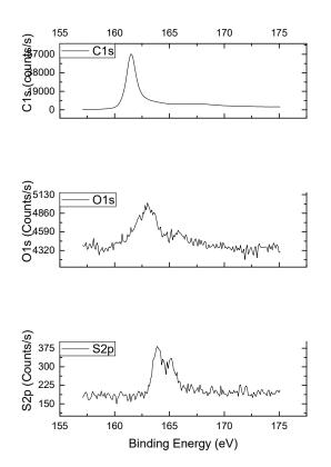
Fig.6. XPS peaks for carbon black nanocomposites
