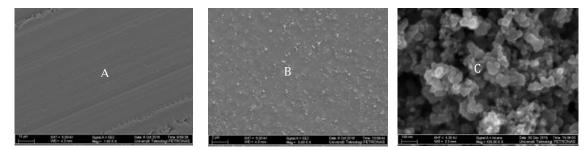
Fig.1. FESEM image of (A) neat epoxy (B) epoxy/CB nanocomposites and (C) CB nanoparticle.
