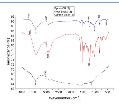
Fig.5. FTIR spectrum of CB, epoxy and nanocomposites
