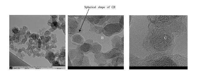
Fig.8. TEM images of CB nanoparticles
