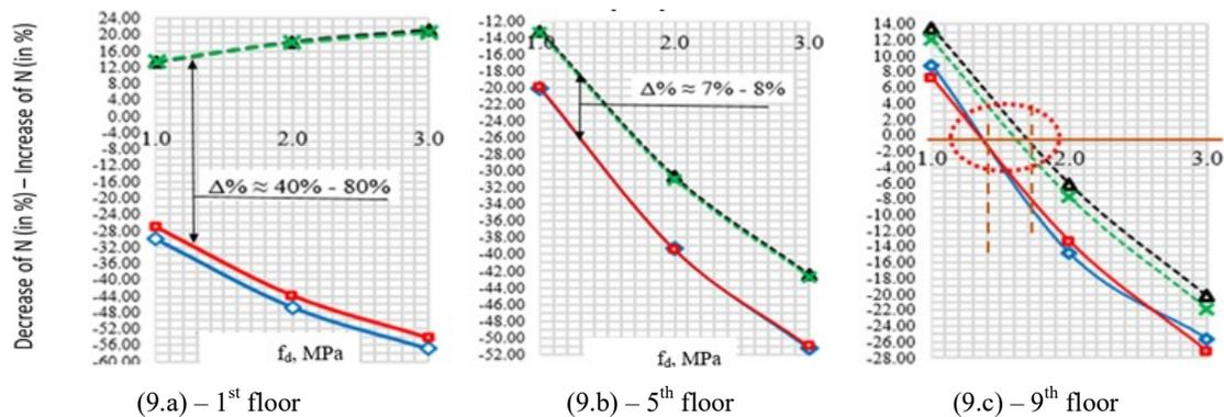
**Fig.9.** Decrease of longitudinal forces in corner columns according to the strength of the masonry infill walls and kind of loading: (a) on the lower floor; (b) on the middle floor; (c) on the upper floor
