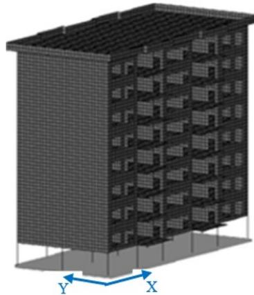
Fig.6. 3D finite element model (model 3) without the masonry infill walls on the ground floor
