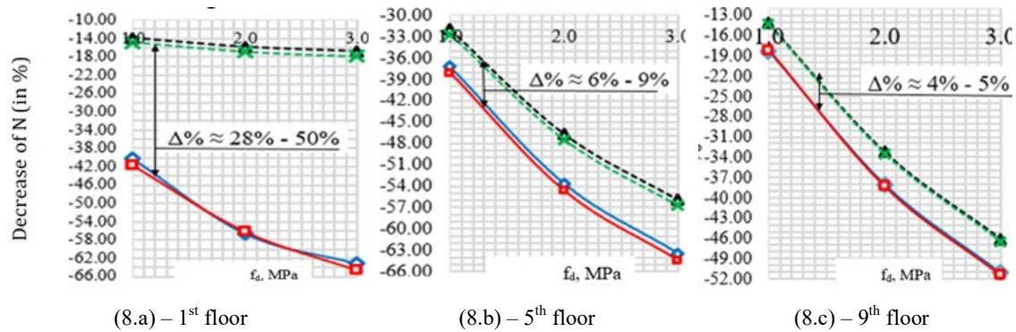
**Fig.8.** Decrease of longitudinal forces in external non-corner columns according to the strength of the masonry infill walls and kind of loading: (a) on the lower floor; (b) on the middle floor; (c) on the upper floor
