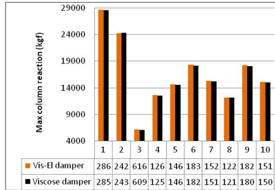
**Fig.7.** Comparison of peak response for collision of two intermediate steel moment frames for two cases of viscoelastic and viscous dampers
