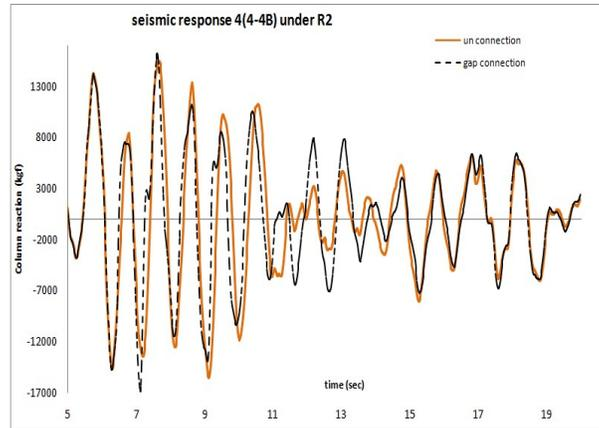
**Fig.2.** Free (-) and pounding-involved (--) Seismic response for collisions an intermediate moment steel frame with adjacent inverted-braced frame under record R2 of table 1.
