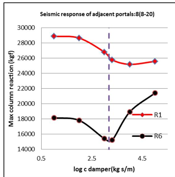
**Fig.6.** Peak response for colliding of an intermediate and a special steel frame for different records vs. damping of damper
