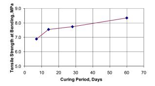
Fig.3. Dependency of the tensile strength at bending on the curing period of HSCAC samples
