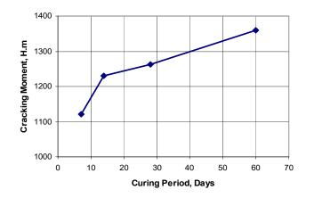
Fig.2. Dependency of the cracking moment on the curing period of HSCAC samples of 100x100x450 mm
