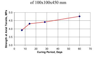
Fig.4. Dependency of the strength at axial tension on the curing period of HSCAC samples of 100x100x450 mm
