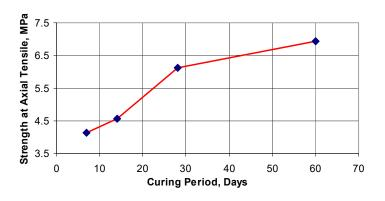
**Fig.4.** Dependency of the strength at axial tension on the curing period of HSFPC samples of 100x100x400 mm
