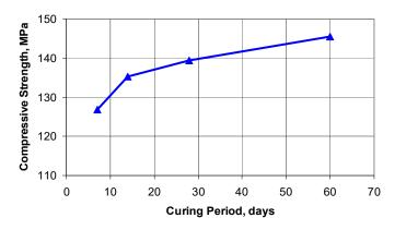
Fig.1. Compressive strength depending on the curing period of HSFPC samples of
