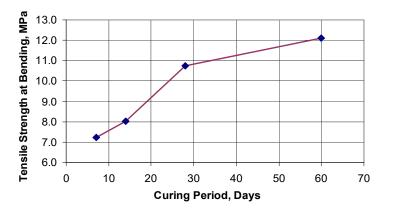
Fig.3. Dependency of the tensile strength at bending on the curing period of HSFPC samples
