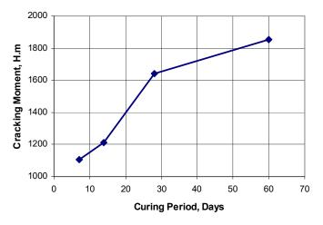
Fig.2. Dependency of the cracking moment on the curing period of HSFPC samples of
