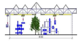
**Fig.2.** The pavilion-type building. The wide-span construction with suspension catheads and a multistoried stack frame where the equipment of smaller sizes can be displayed. Demountable metallic constructions permit the dismantling and reassembling of the stack frame in any
