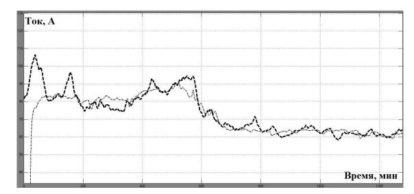
Fig.4.Results of modeling of unit's operation, using Kolmogorov-Gabor polynomial
