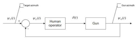
**Fig.1.** The block diagram of the control system of artillery turret <sup>[7]</sup>
