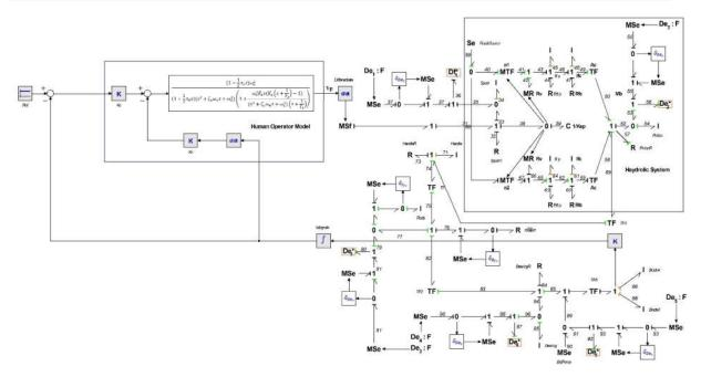
Fig.8. Bond graph model of the collective control of the system with LFT model
