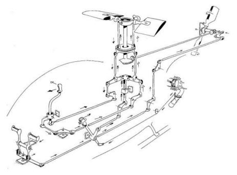
Fig.4. Schematic of collective and cyclic control system of helicopter
