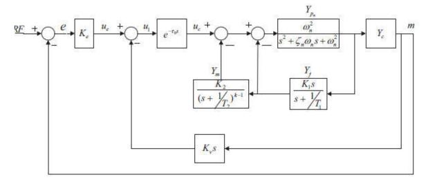
Fig.3. Hess structural model of the human operator
