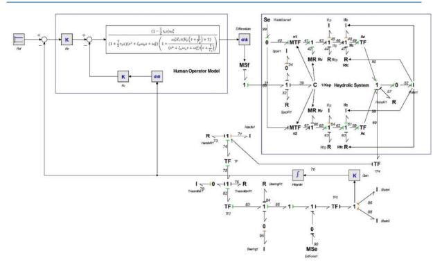
Fig.5. Bond graph model of collective control system of helicopter
