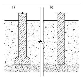
Fig.1. Scheme of bored pilesa) with widened base; b) without widened base
