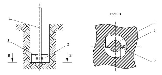
**Fig.3.** Dipping the equipment into the Soil 1 - barrel; 2 - pointed plates; 3 - welded joints
