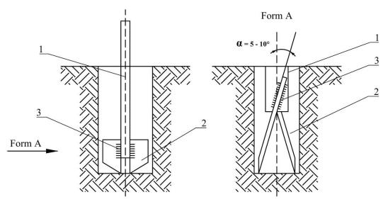
**Fig.2.** Dipping the equipment into the Soil 1 - barrel; 2 - pointed plates (thickness = 3-4 mm); 3 - welded joints
