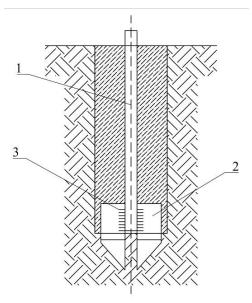
**Fig.4.** Bored pile after the borehole concreting 1 - barrel; 2 - pointed plates; 3 - welded joints
