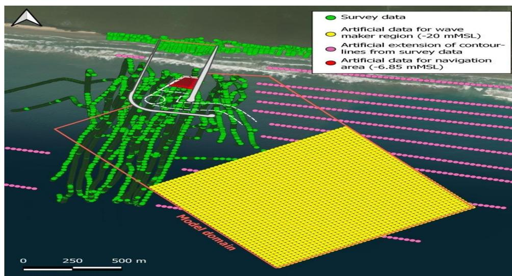
**Figure 4** Types of bathymetric data used in the seven models (present figure show Case 1)
