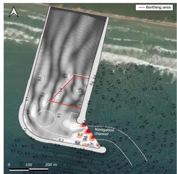
Figure 12 Case 2 wave disturbance coefficient
