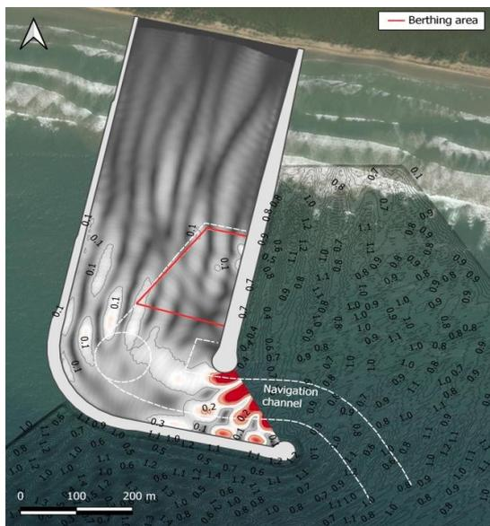
Figure 11 Case 1 wave disturbance coefficient
