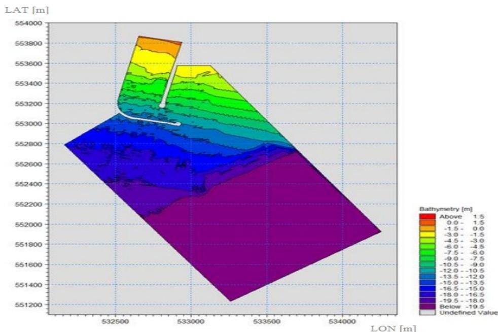
Figure 7 Example of the model domain and bathymetry for the three models (present figure depicts Case 1)
