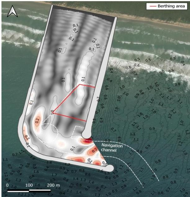
Figure 13 Case 3 wave disturbance coefficient
