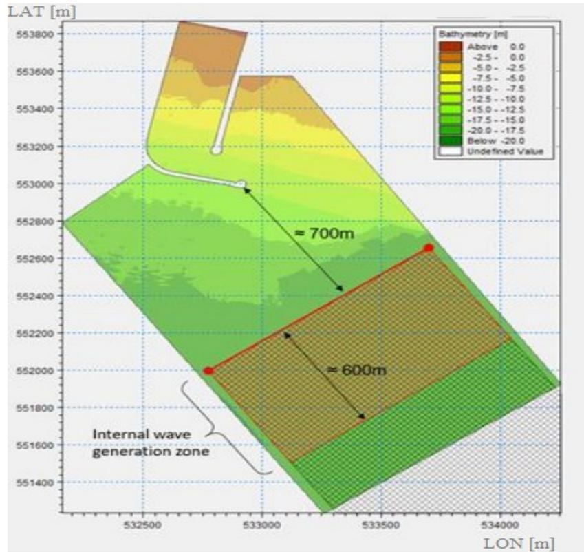
Figure 9 Example layout of internal wave generation zone (present figure shows Case 1)
