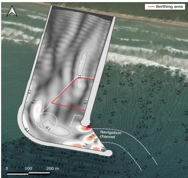
Figure 17 Case 7 wave disturbance coefficient
