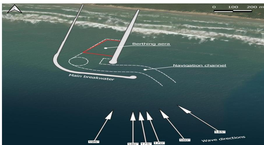
Figure 3 Overview of the project area and simulated wave directions.
