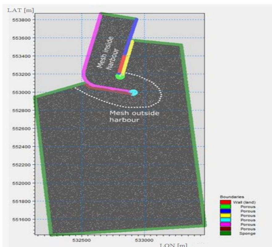
**Figure 8** Example of model boundaries (present figure shows Case 4)
