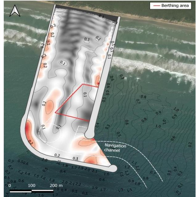
Figure 16 Case 6 wave disturbance coefficient
