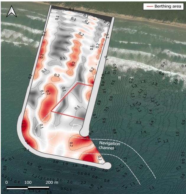
Figure 15 Case 5 wave disturbance coefficient.
