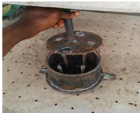
Figure 5 Assembled briquette mould
