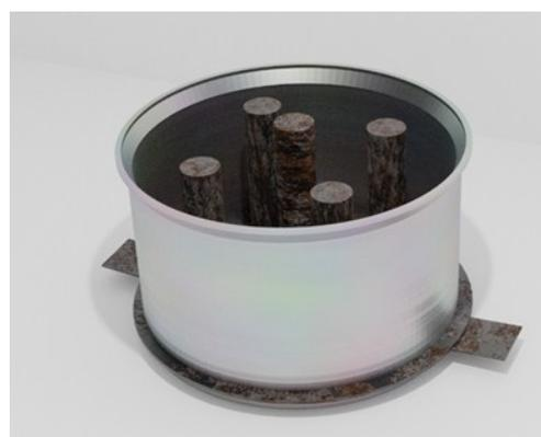
(f) Assembly of Briquette mould
