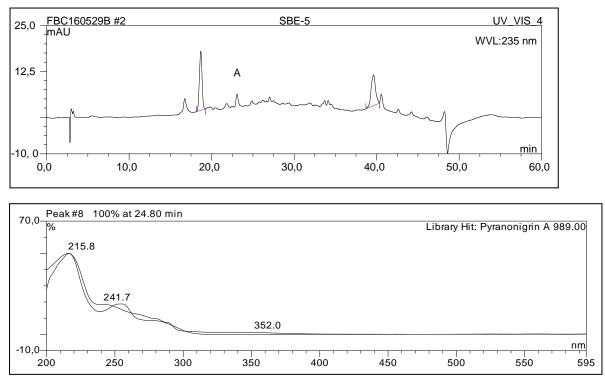
**Figure 1:** HPLC Chromatogram of SBE 5 (6:4), correlation  $\ge$  987 **KEY; A**- Pyranonigrin A Hit 989.00 (Rt = 24.80 min)
