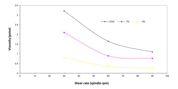
Fig 2: Effect of shear rate on the viscosity of calamine suspension formulated with 2 % w/v of various suspending agents
