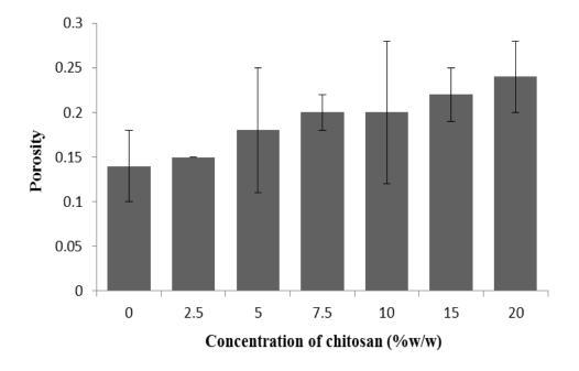
Figure 1: Plot of porosity versus concentration of chitosan
