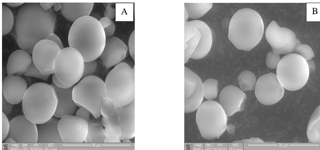
**Figure 1: SEM of native *M. esculentus* starch (A) and oxidized *M. esculentus* starch (B)**
