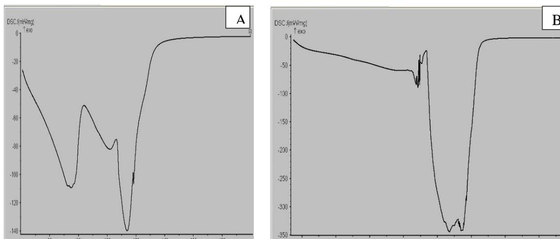
**Figure 3: DSC thermogram of native *M. esculentus* starch (A) and oxidized *M. esculentus* starch (B)**
