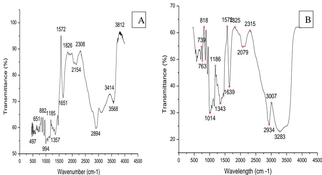
**Figure 5: FTIR Spectrum of native *M. esculentus* starch (A) and oxidized *M. esculentus* starch (B)**
