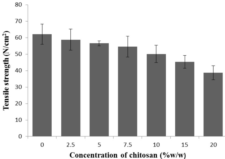
**Figure 2: Plot of tensile strength versus concentration of chitosan**
