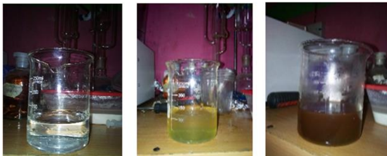
Figure 1. Colour change signifying AgNps synthesis. (A) is clear AgNO 3 solution, (B) is Moringa aqueous extract and (C) is synthesized silver nanoparticle solution
