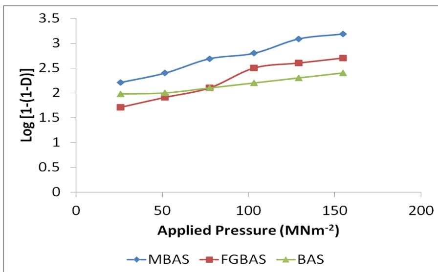
Figure I: Heckel Plot for the native and modified Borassus Starches
