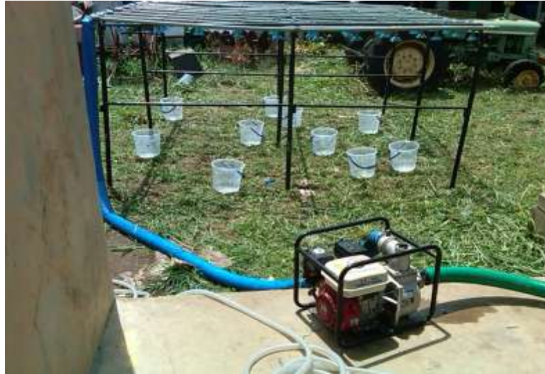
Figure 2 Pump for pumping water into the rainfall simulator
