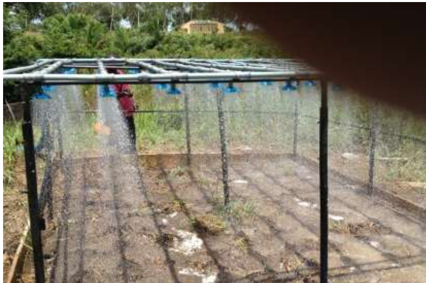
Figure 3 Rainfall simulator in operation on a bared soil
