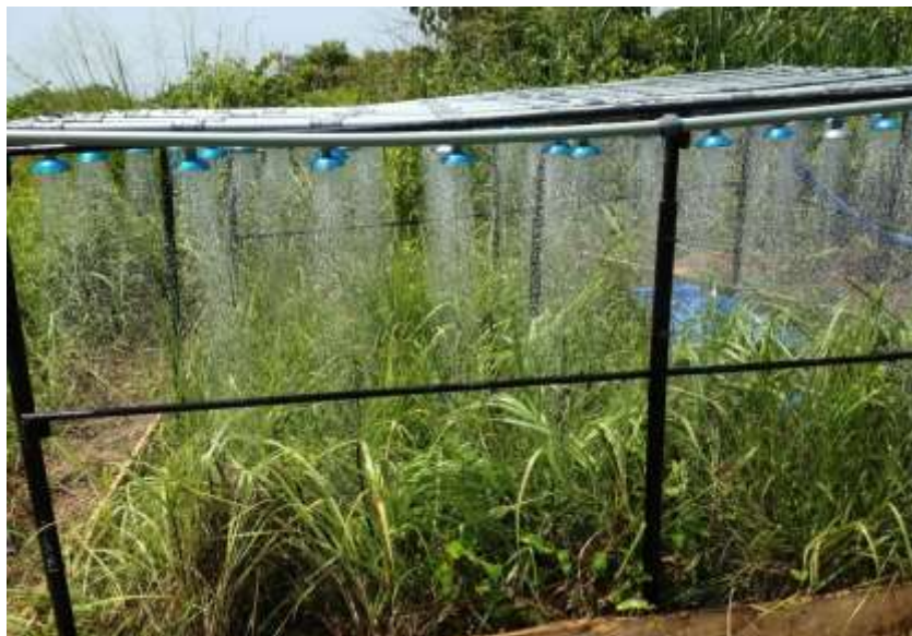
Figure 4 Rainfall simulator in operation on a vegetative cover soil
