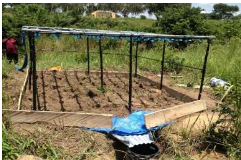
Figure 1: Rainfall simulator and drum in the pit on a bared soil for runoff and soil sediment
