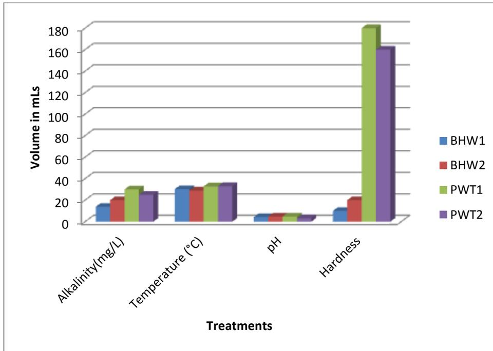
**Figure 2: Physicochemical properties of water samples from boreholes and public water taps in Choba**
