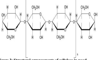
Figure 3: Structural arrangements of cellulose in wood. Source: (Bowyer and Smith 1998).
