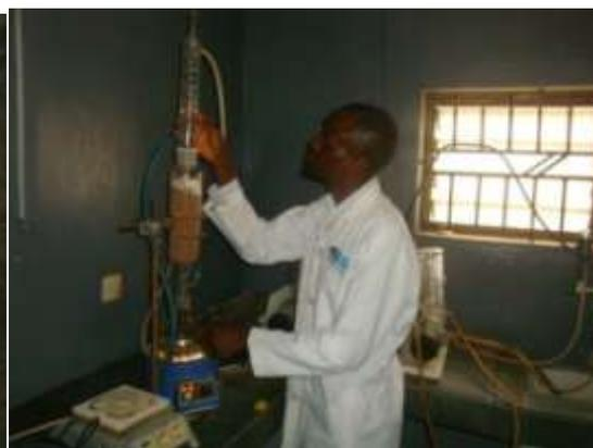
Plate 4: Oil extraction using soxhlet apparatus
