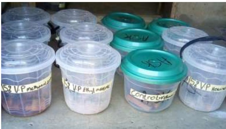
Plate 1: Wood samples soaked in crude extracts for treatment
