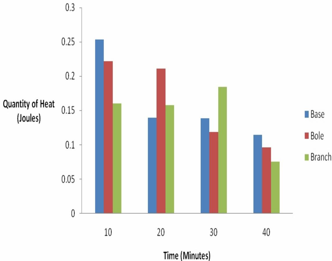
Fig.1.0 Quantity of heat produced (in joules) from *prosopis africana* charcoal samples with time.
