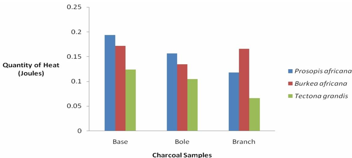
Fig.4.0 The quantity of heat produced (in joules) between charcoal samples.
