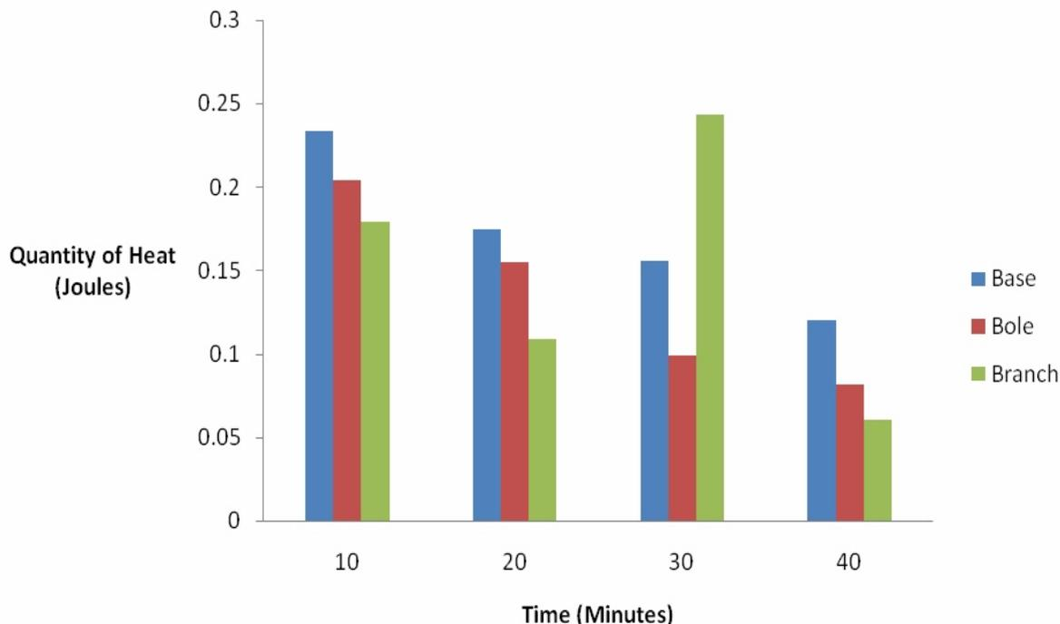
Fig 3.0 Quantity of heat produced (in joules) from *Burkea africana* charcoal samples with time.
