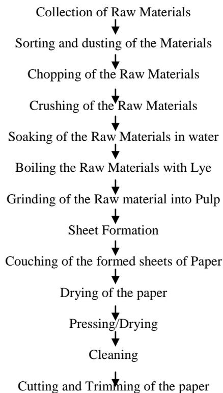
**Figure 1. Chart showing the production Process of Paper from Non Wood Raw Materials**
