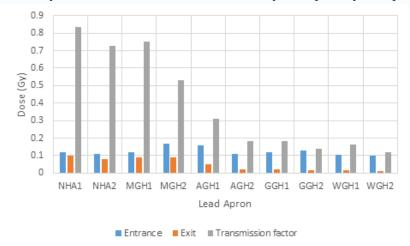
Figure 1: Comparison between Entrance, Exit and Transmission factor
