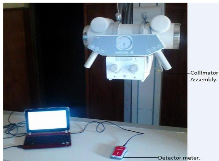
Figure 1: Setup for Measurement of Half Value Layer
