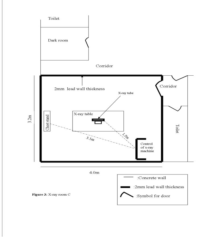
**Figure 3:** Layout of x-ray room C
