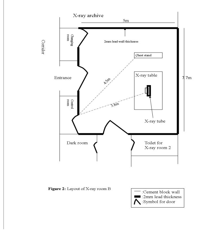
Figure 2: Layout of x-ray room B
