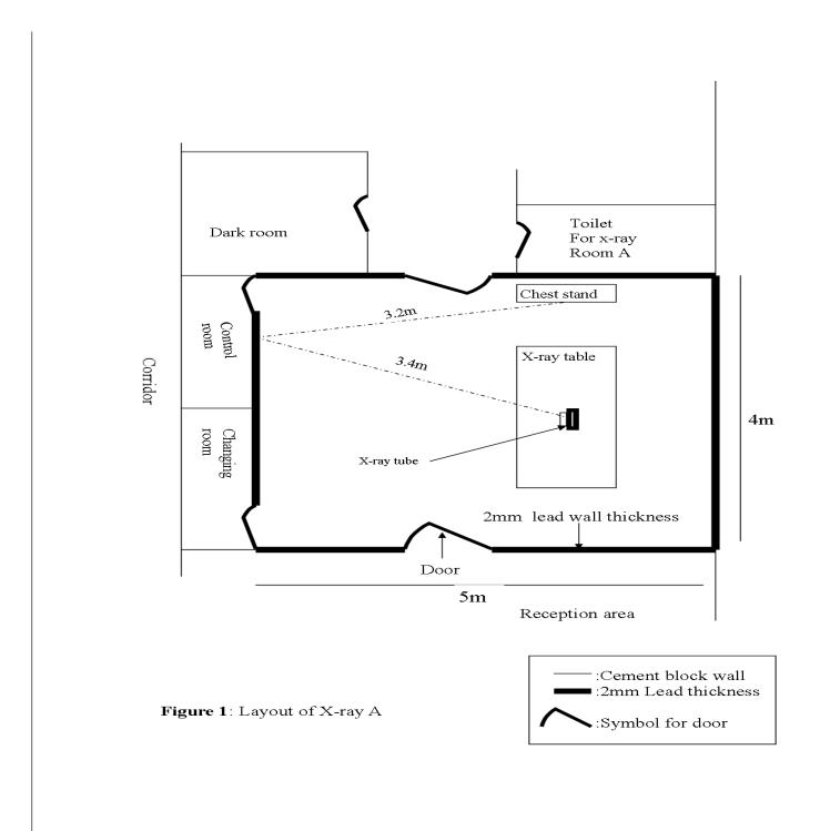
Figure 1: Layout of X-ray room A
