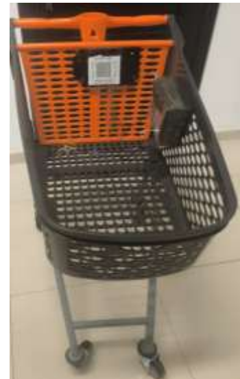
Figure 10: Fully assembled hardware system mounted on the trolley
