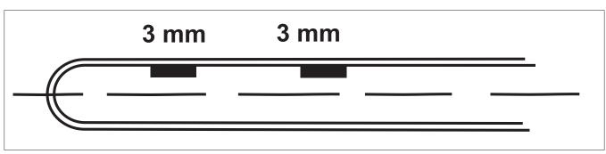
Figure 1: The distal end of the catheter with two slots of 3 mm, one after another
