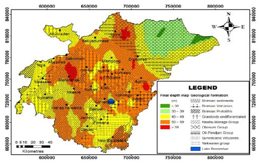
Fig. 3: Overlay of borehole depth on geology
