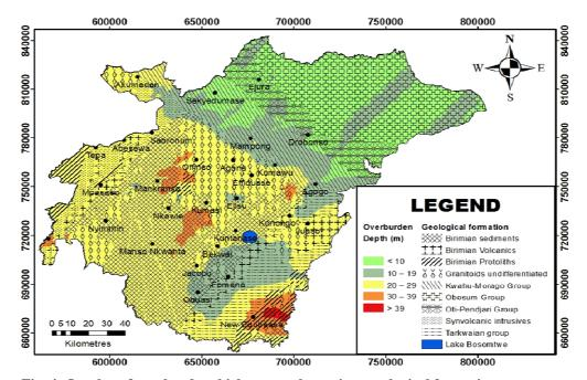
Fig. 4: Overlay of overburden thickness on the various geological formations
