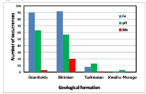
Fig. 7: Major poor water quality parameters in the geological formations
