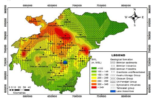
Fig. 5: Overlay of SWL elevation on the geology
