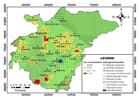
Fig. 8: Overlay of iron concentration on geological formation
