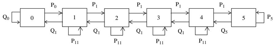
**Fig. 1: The transition diagram of a finite state birth-death process with  $N = 5$**
