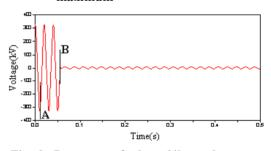
Fig. 6: Permanent fault at 64km voltagemaximum
