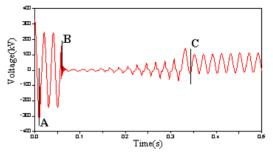
Fig. 4: Transient fault at 64km voltagemaximum
