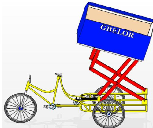
**Fig. 8: Model of existing tricycle with mechanism in place as lift-tilt position**
