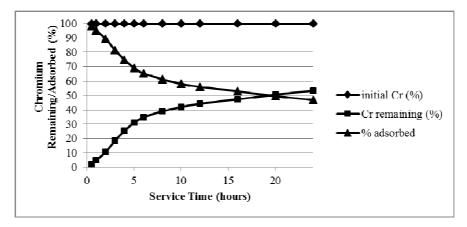
Fig. 3 :Effect of time on chromium adsorption at bed height of 4 cm (Carbon = Local 1:2, initial chromium = 3.151 mg/L)
