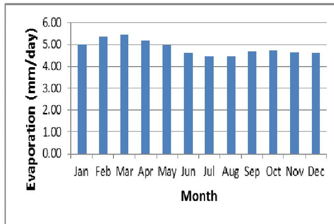
Fig. 12: Estimated average monthly evaporation for Kumasi using the Penman Evaporation Model (2001-2010)
