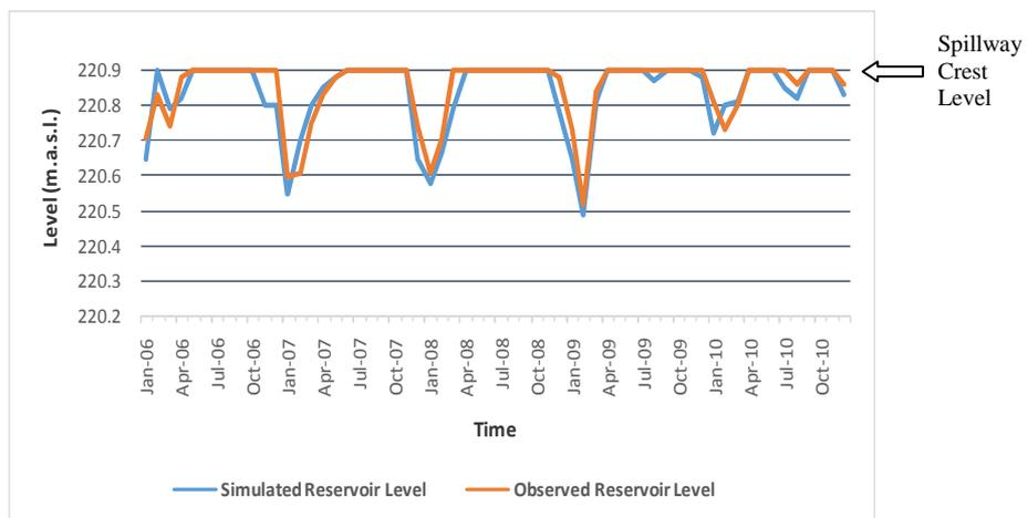
Fig. 14: Simulated and observed reservoir levels for the validation period (2006-2010)
