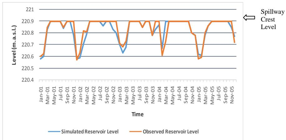
Fig. 13: Simulated and observed reservoir levels for the calibration period (2001-2005)
