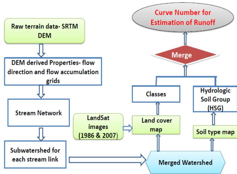
Fig. 4: Procedure for catchment delineation and derivation of curve number
